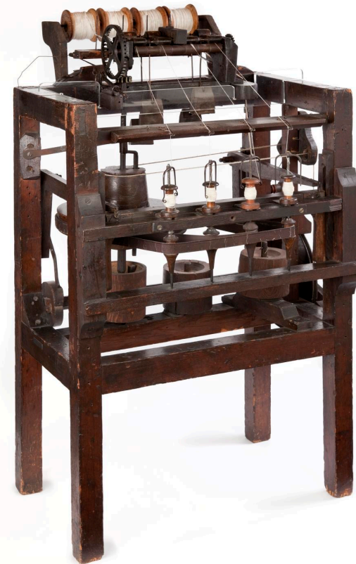
Spinning engine by Arkwright. Water powered. Research by Arkwright and his team of clockworkers from 1767 to 1771. Patented.
